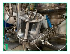
Attach sight glass to extractor's sanitary flange connections
