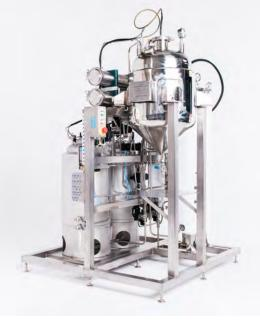
HEATING: Recirculating Water Heater 9kW PROCESS TEMPERATURE RANGE: -65°C to 0°C PRESSURE RATING: 250PSIG REACTOR CAPACITY: 32L liquid (43L total) 28L plant feedstock CYCLE TIME: 50 minutes (recipe dependent) THROUGHPUT: 18 lbs dry feed stock, 25 lbs wet
